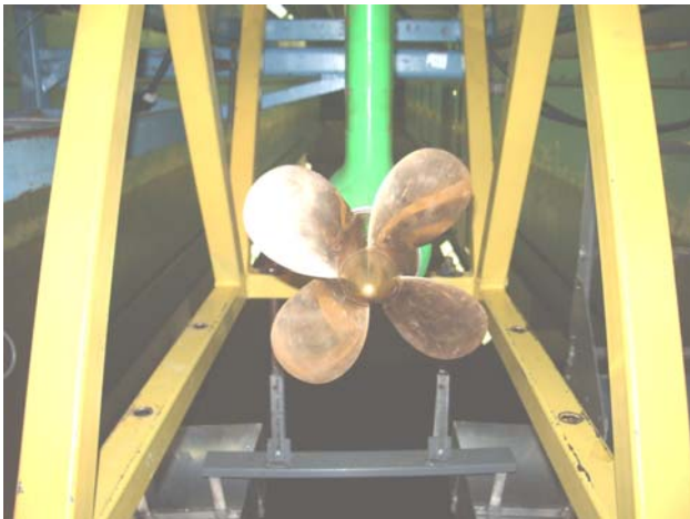
(c) Average Pod 01: The pod is attached with the NSERC-NRC dynamometer before the test started (Front View).
