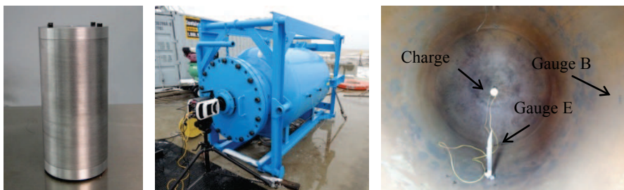
FIGURE 3. Experimental setup: HIPed 10\text{Al} + \text{MoO}_3 cylinder casing assembly (left); 2.1 \text{ m}^3 cylindrical explosion chamber (middle); cylindrical symmetry test configuration (right).
