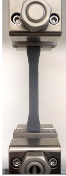
Fig. 3: Uniaxial tensile tests of 3D-printed dogbone samples.
