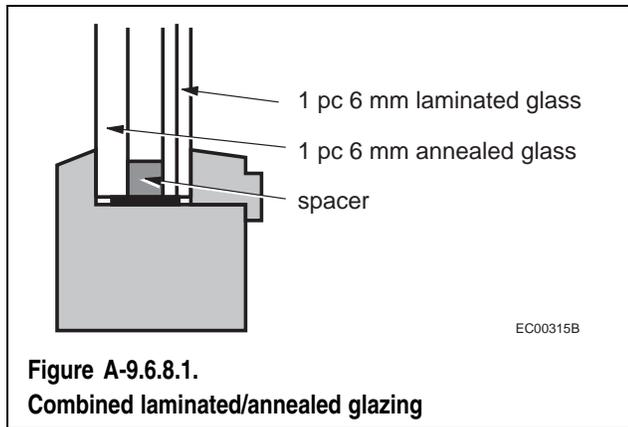
Laminated glass is more expensive than annealed glass and must be used in greater thicknesses. Figure A-9.6.8.1. shows an insulated sidelight made of one pane of laminated glass and one pane of annealed glass. This method reduces the cost premium that would result if both panes were laminated.
