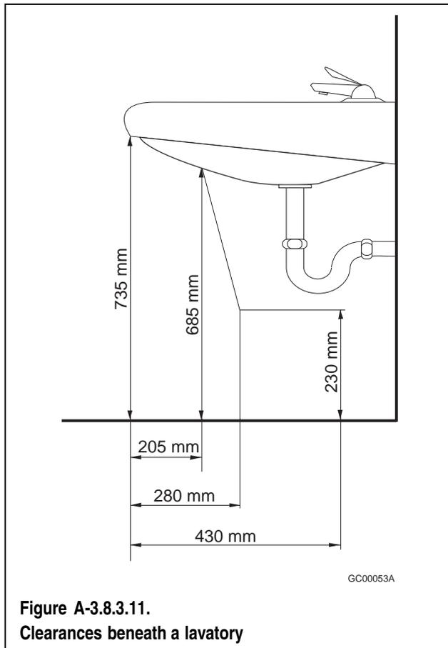
**A-3.8.3.11.(1)(d) Pipe Protection.** The pipes referred to in Clause 3.8.3.11.(1)(d) include both supply and waste pipes. The hazard can be prevented by insulating the pipes, by locating the pipes in enclosures, or avoided by limiting the temperature of the hot water to a maximum of 45°C.
