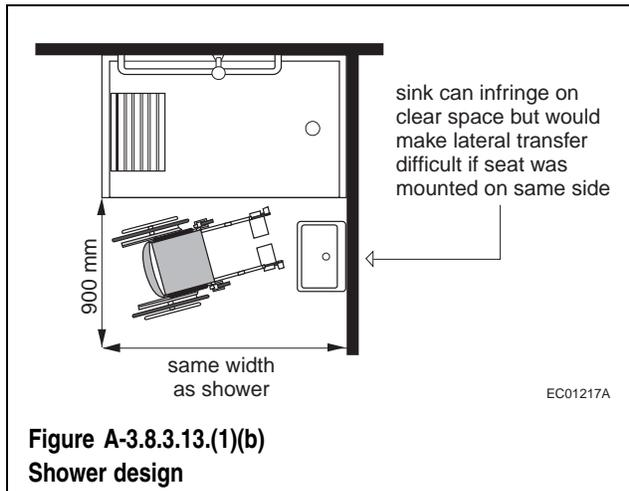
**A-3.8.3.13.(1)(f) Grab Bars.** One horizontal grab bar is required to be installed on the wall next to the seat. A grab bar behind the seat would prevent the user from leaning back against the wall, while one located on the wall opposite the seat cannot be reached from the seated position. The seat itself may be used in conjunction with the bar for transfer. If design flexibility is required, fold away grab bars can be used as an alternative.
