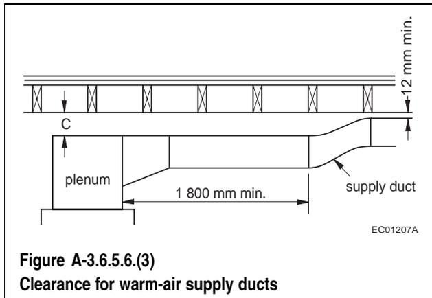
**A-3.6.5.6.(4) Clearance for Warm-Air Supply Ducts.** Applicable to forced-air furnaces where permissible clearance C above plenum is more than 150 mm.
