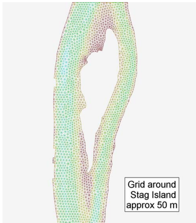
Figure 2 - Example of detailed island in the finite element grid
