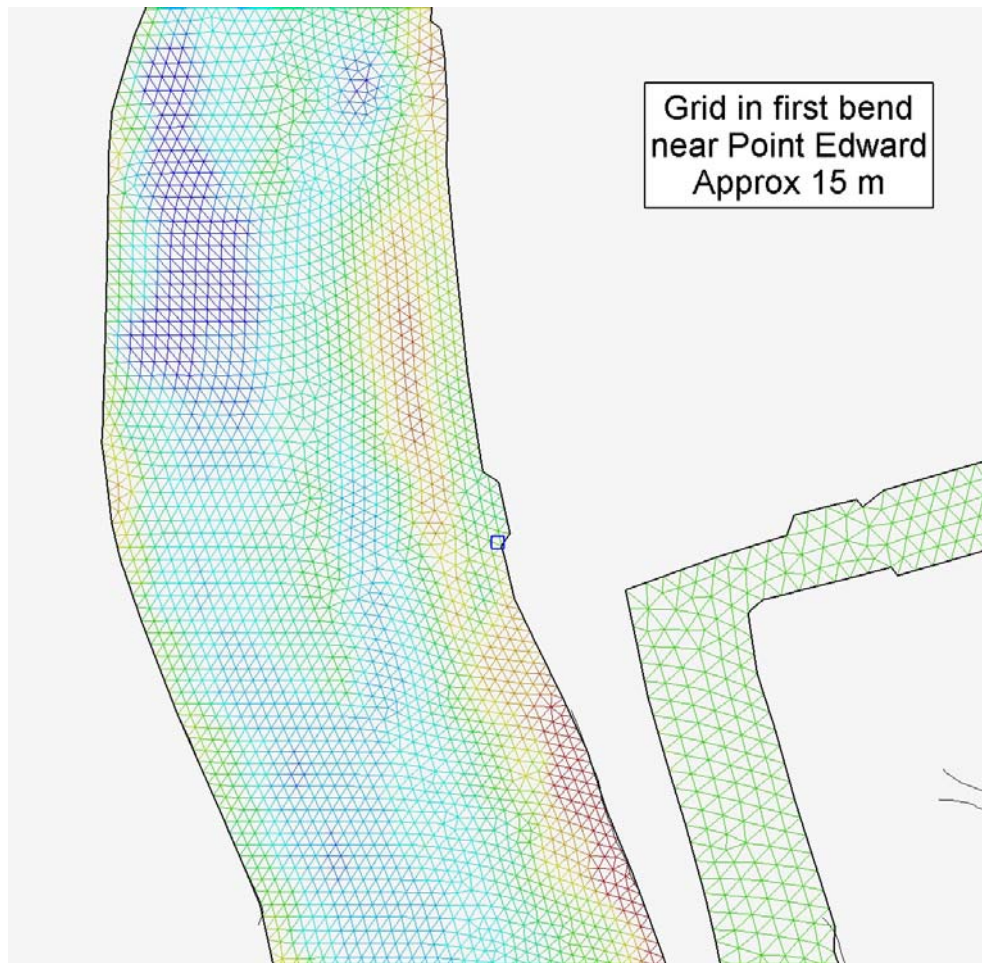
Figure 3 - Example of fine grid detail
