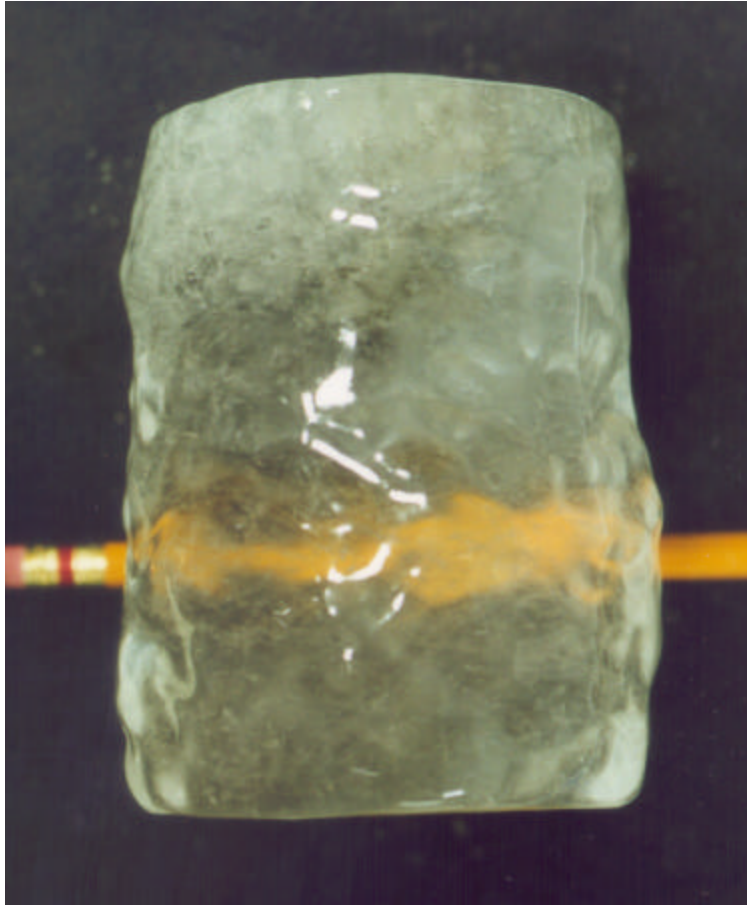
Figure 26: Ice specimen from laboratory-produced ice tested at high confinement. The pencil can be seen through the ice, a feature that is characteristic of strongly recrystallized ice that displays very little microcracking. The lighter zone near the upper surface is caused by the presence of air entrapment in the specimen before deformation.
