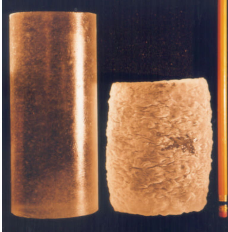
Figure 21: Ice specimens made from laboratory-produced ice. Initial size for all specimens (both this ice and iceberg ice) was 155 mm in length and 70 mm in diameter (the pencil is for scale). Left, undeformed; right, deformed to 33% true strain at 50 MPa confinement and -10^{\circ}\text{C} . Note the final barrel-shape configuration.
