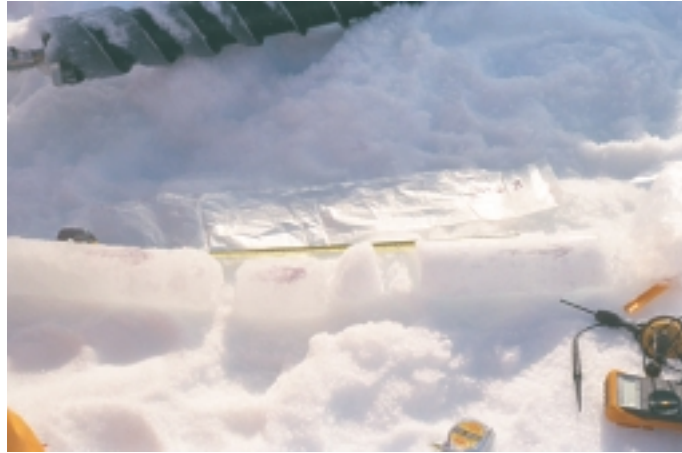
Figure 36 Core of the consolidated layer of ice from Site 8 that was retained for crystallographic studies
