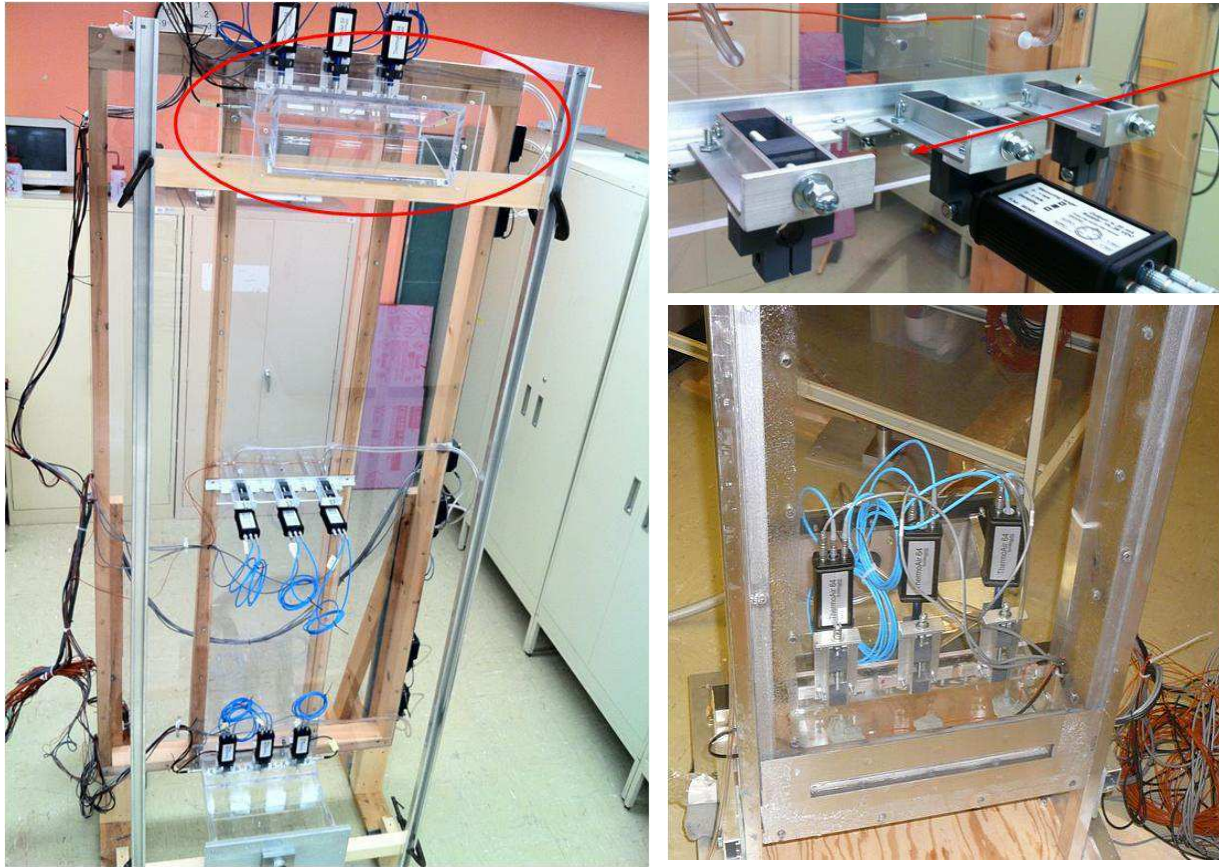
Figure 4 – Location of anemometers at each of the control locations of the cavity air flow characterization apparatus; at inlet and outlet chutes and at mid-height of cavity space
