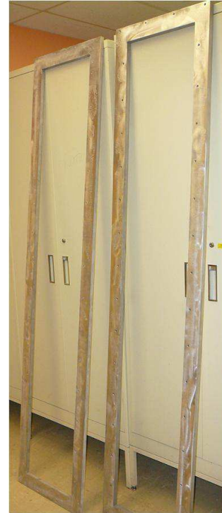
Figure 7 – Photo showing metal spacers for cavity depths of 10, 20 and 25 mm
