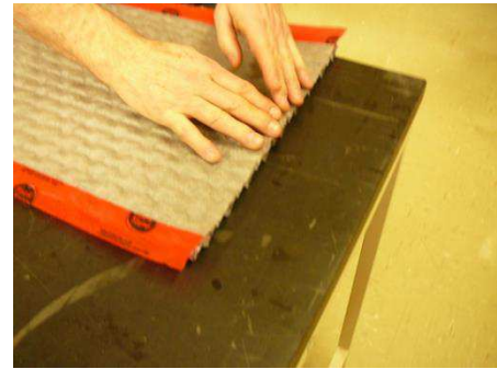
Figure 29 – Dimpled plastic membrane and parging screen fabric showing: (A) flow of air between dimpled membrane and parging fabric; (B) Specimen fabrication
