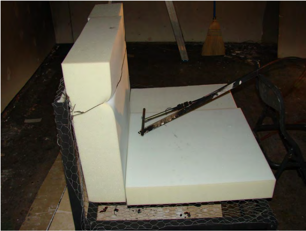
Figure 5. Mockup sofa arrangement for Tests 2-6.
