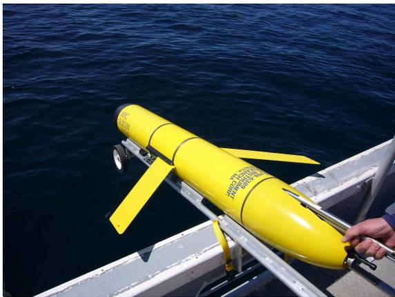
**Figure 2:** Launching a glider over the side of a small fishing vessel
