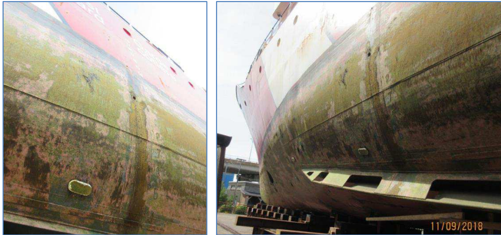
Fig.12: Images of port side of hull during September, 2018 dry dock. The level of fouling is similar to that encountered in May, 2018.
