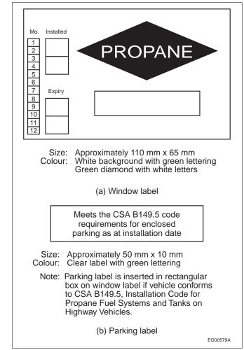
Figure A-2.4.4.5.(1) Propane fuelled vehicle window and parking labels
