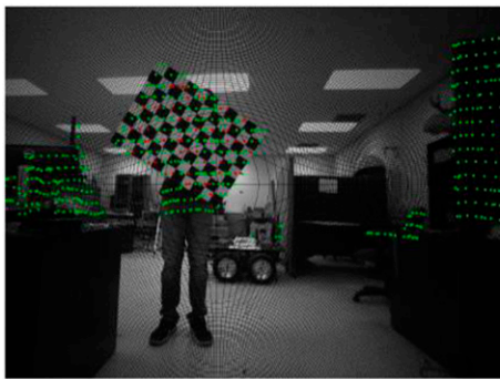
(a) Matlab LiDAR calibration verification by projecting the point cloud on the image.
