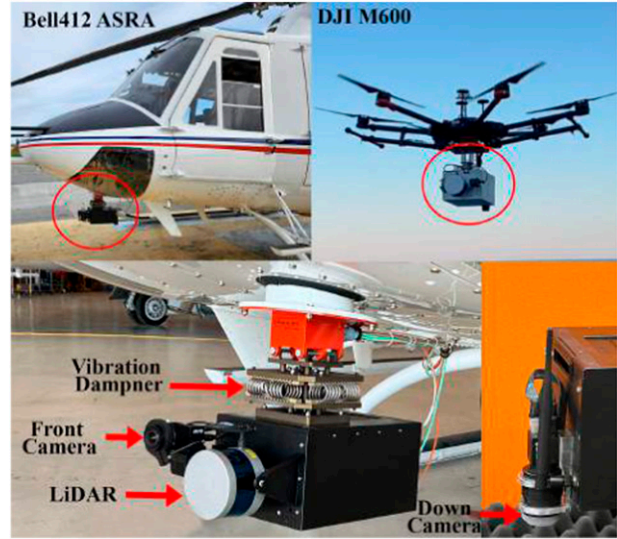
Figure 1. MUN Sensor Payload Flight Test Configurations: NRC Bell 412 ASRA Nose Mount (Top/Bottom Left); MUN DJI-M600 air-frame mount top right.
