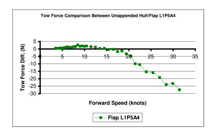
Figure 8: Relative Tow Force With/Without Flap Fitted
