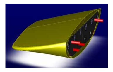
Figure 10: Final Flap Design for the Physical Model
