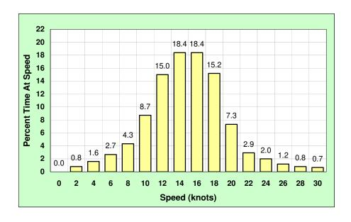
Figure 9: HALIFAX Class Frigate Peace Time Percent Time at Speed Profile
