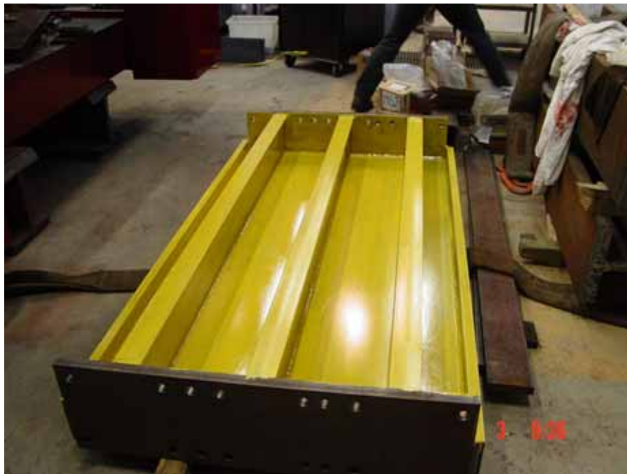
Figure 8. Small grillage ready for application of strain gauges.
