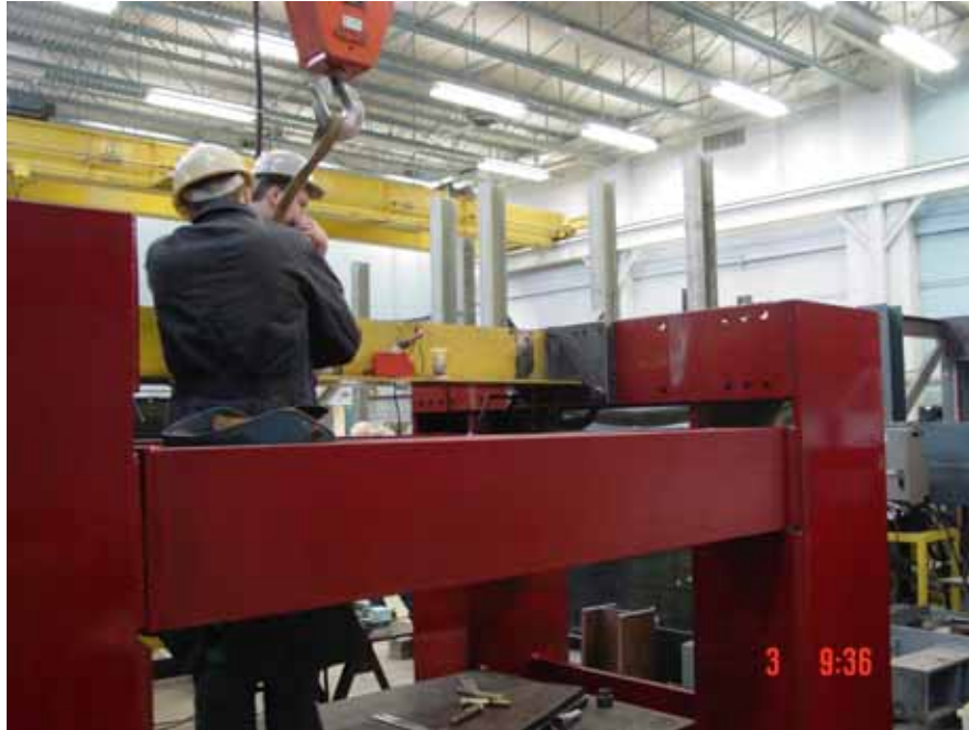
Figure 7. Preparations for testing final single frames in the grillage support frame.
