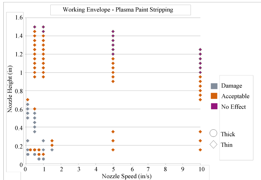
Figure 5. 2D graph of damaging, acceptable and ineffective limits using 3 passes of the plasma pen.
