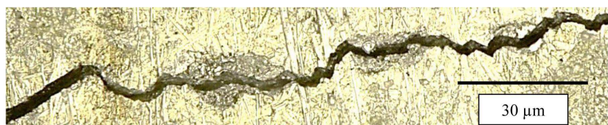
Figure 8. Close-up view of a fatigue crack in an aluminium panel section, showing almost no visible debris after plasma paint stripping.
