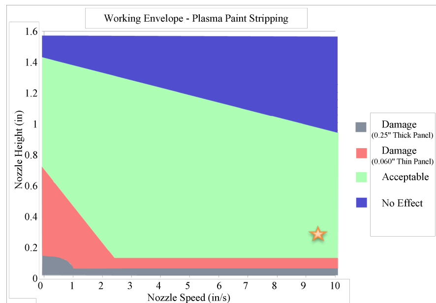
Figure 6. Map of effective (acceptable), damaging and ineffective parameters for the paint stripping machine on the specified paint scheme. The star indicates the selected parameters that were used in the comparative study.
