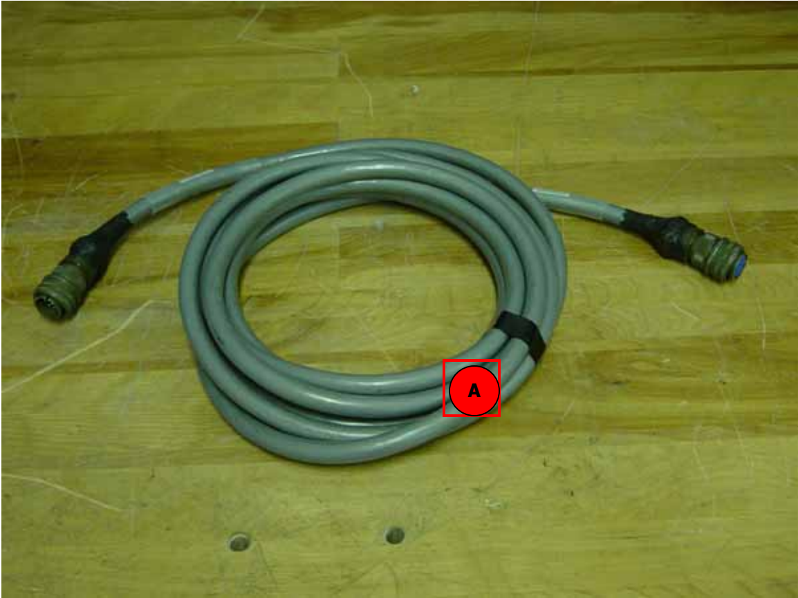
Figure 15. Power Enclosure to Computer Enclosure Cable.
