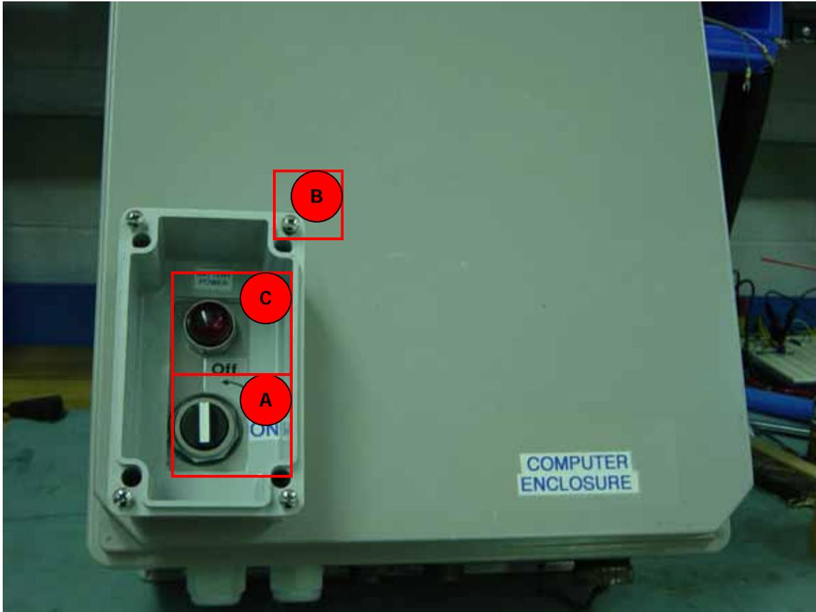
Figure 6. Battery UPS Switch.
