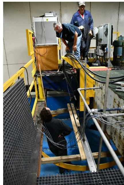
Figure 48: The carriage has been move to the location of a test. Below it is the instrumentation used to monitor the ice loading event and the ice response. Person with orange jacket for scale, upper right.
