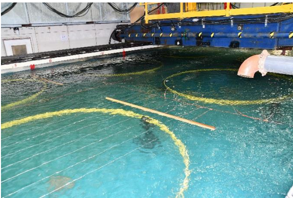
Figure 41: The eight circular test frames (yellow) are deployed inside the ice tank. The person at far back is for scale.
