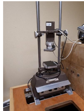
Figure 17: The un-instrumented Chatillon-type test frame (see Figure 18 for scale).
