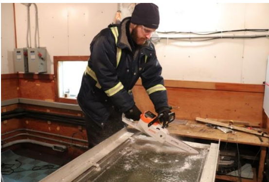
Figure 7: Beam extraction from the growth basin.
