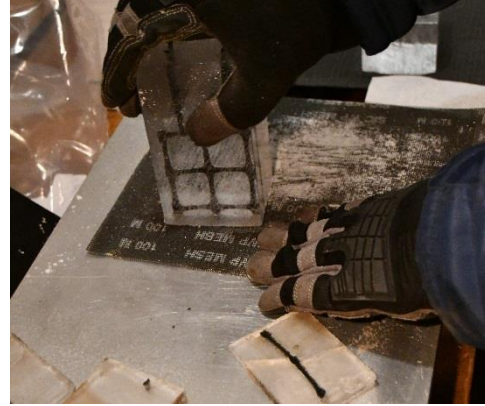
Figure 26: The band saw surface is smoothed on a 100 grit sanding mesh.
