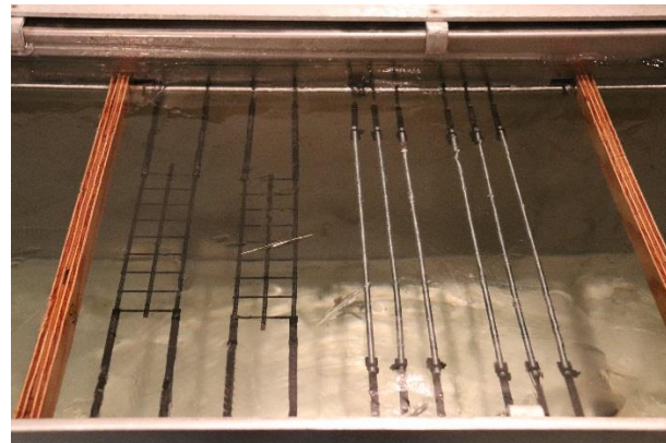
Figure 6: Set-up of reinforcement in the basin prior to bringing water into the basin. In this picture, the Stratagrid SG150 (left) and the threaded rods (right) are shown – these are discussed later.
