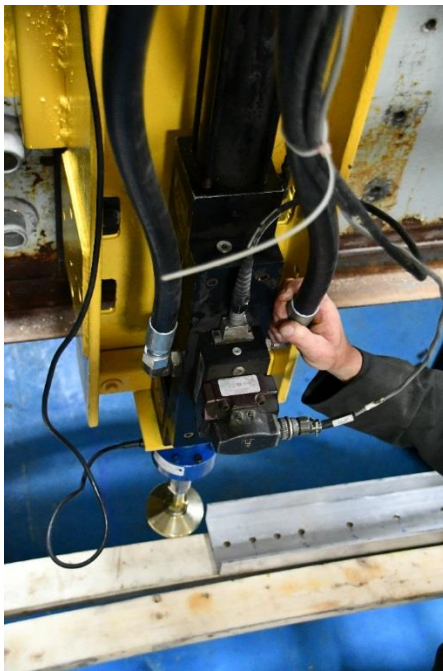
Figure 49: Piston viewed from above. The circular platen (stainless steel) at its end can be seen below the (blue) load cell.
