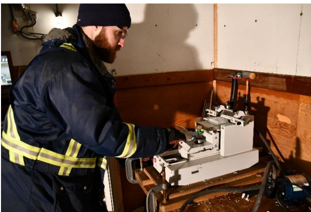
Figure 29: The glass plate and the ice slice are installed onto the microtome.
