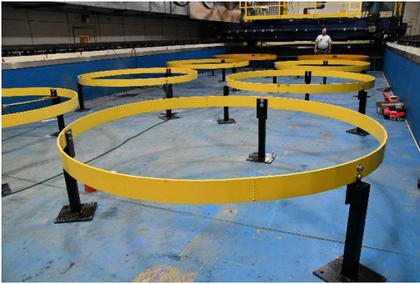
Figure 41: The eight circular test frames (yellow) are deployed inside the ice tank. The person at far back is for scale.
