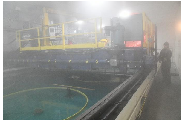
Figure 44: 'Seeding' event at 15°C – the mist in the air is made from tiny crystals that settle on the water surface and initiate ice growth.
