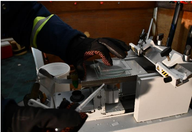
Figure 31: The ice/glass assembly is then flipped upside down onto another clean glass plate (i.e. with the microtomed surface against it), and while applying a slight downward pressure on it, a bead of water is run along the full perimeter (using a plastic eye dropper).
