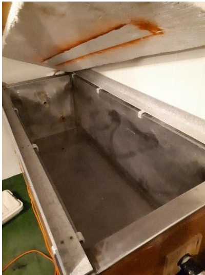
Figure 5: Growth basin (1600 mm in length, 600 mm in width).
