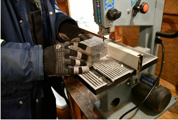
Figure 25: A test beam is cut with a band saw.
