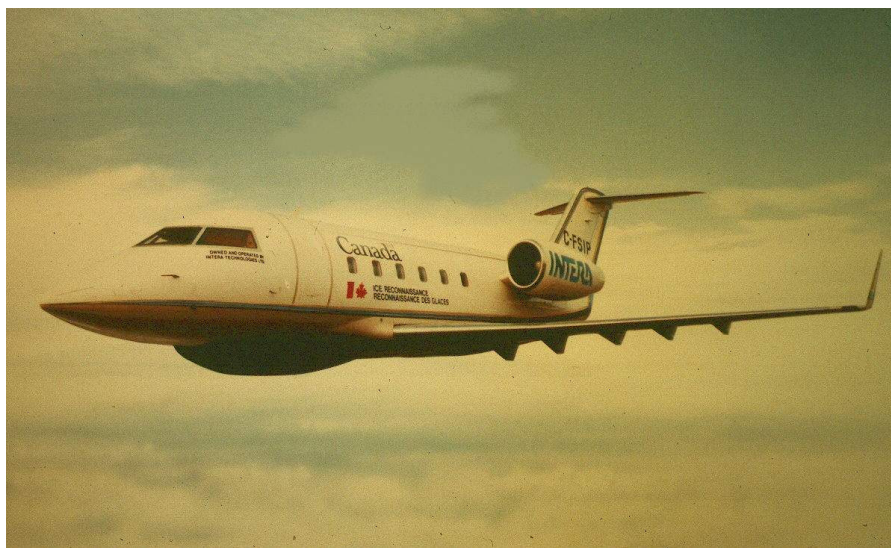
Figure 6: CIRS SAR-equipped ice reconnaissance aircraft
