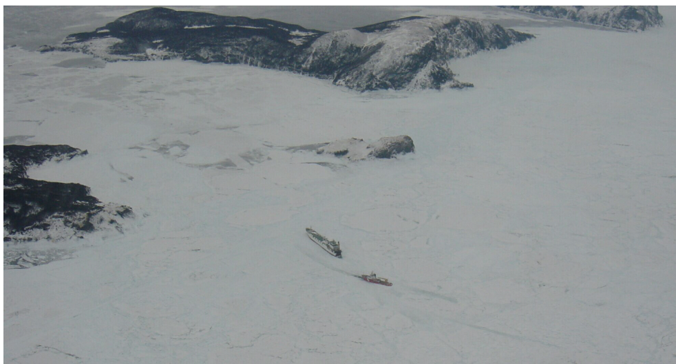
Figure 24: Photograph showing an icebreaker attempting to free a vessel beset in ice under pressure.
