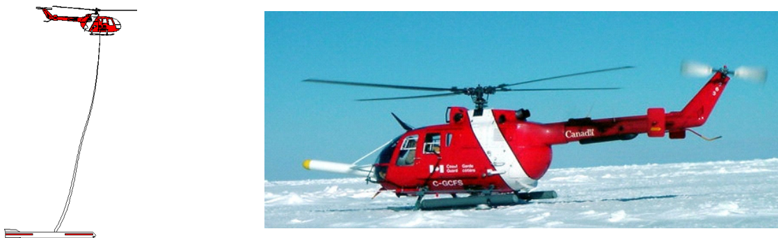
Figure 28: Illustration of the fixed mount ice thickness sensor
