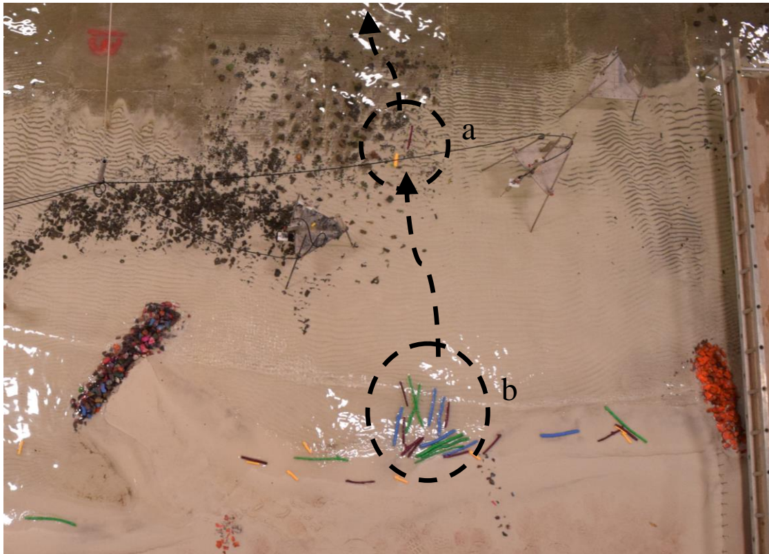
Figure 5. Snapshot showing effects of wave-driven circulation on debris transport.
