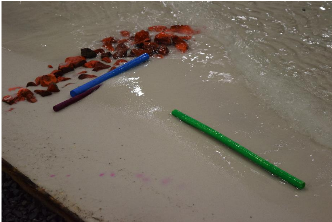
Figure 7. Debris partially buried by silica sand.
