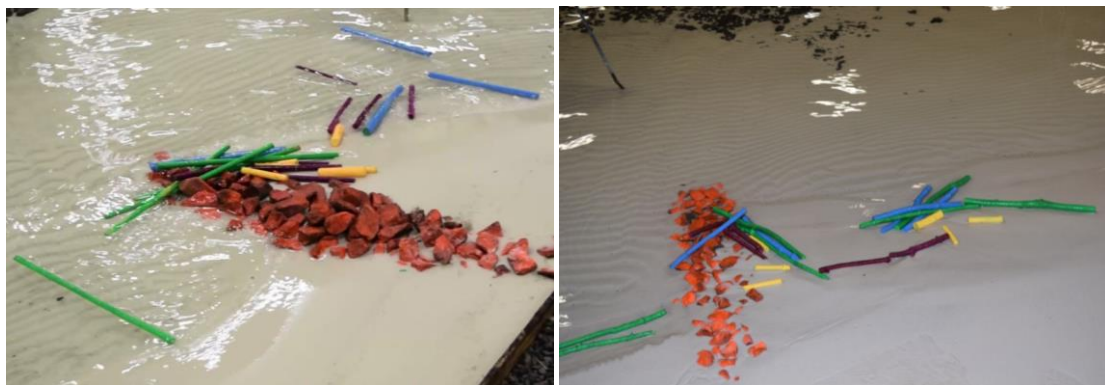
Figure 2. Model woody debris: dowels (left) and tree branches (right).
