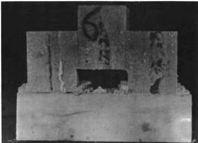
Photo No. 10. Welded shear test specimen, before test. See Table 15.
