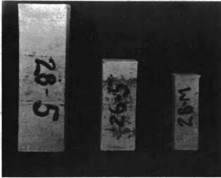
Photo No. 14. Test specimens for plastic flow in compression. At left - 28-5 - 4 by 4 by 12 in. for loading perpendicular to frozen surface, 26-5 is about 2.8 by 2.8 by 7 in. and 28-M is 2 by 2 by 6 in.
