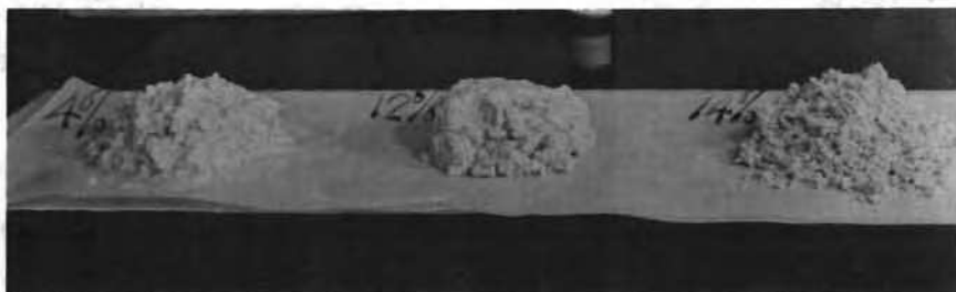
Photo No. 26. Showing appearance of 4, 12 and 14 per cent pulp. Note water which has drained from 4 per cent specimen.
