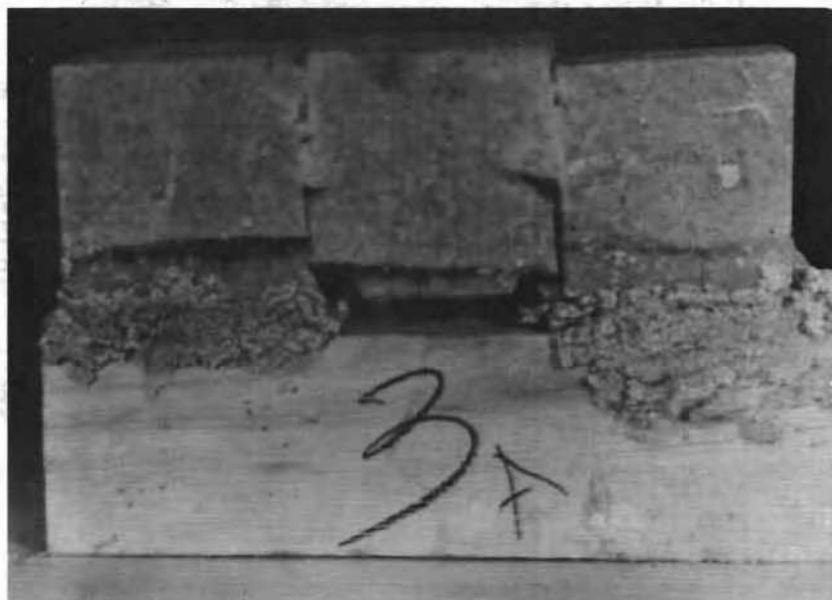
Photo No. 11. Shear of homogeneous pulp without welds. As shown specimen was still carrying about 80 per cent of maximum load. What appears to be saw cut at top, right side, is vertical face of centre portion which was above level of portion to its right at start of test. See Table 16.
