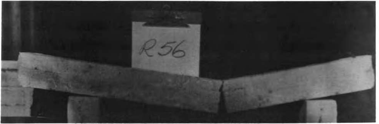
Photo No. 16. Beam reinforced with \frac{1}{4} -in. round steel rod. Note hook at right end has been pulled into beam. Upper surfaces plane from ends to fracture. Loaded at one third points, beam in this condition was carrying a greater load than at test failure.
