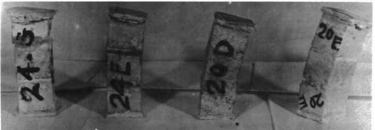
Photo No. 15. Typical appearance of 2- by 2- by 6-in. compression pieces after test. Bending stresses increase rapidly as specimen begins to deform and buckle.
