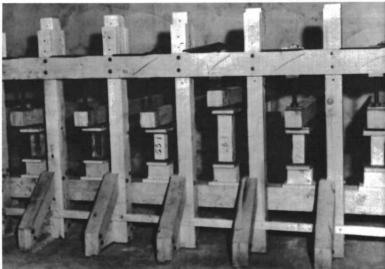
Photo No. 8. Compression specimens. Left to right, river ice loaded to 50 and later 75 psi. Specimen 53-1 is reinforced with wood; 28-1 is 4 per cent pulp carrying 100 psi and specimens at right are of 6 per cent pulp carrying 200 psi. Three specimens at right are covered with waxed paper to prevent evaporation. See Tables 21 and 22.
