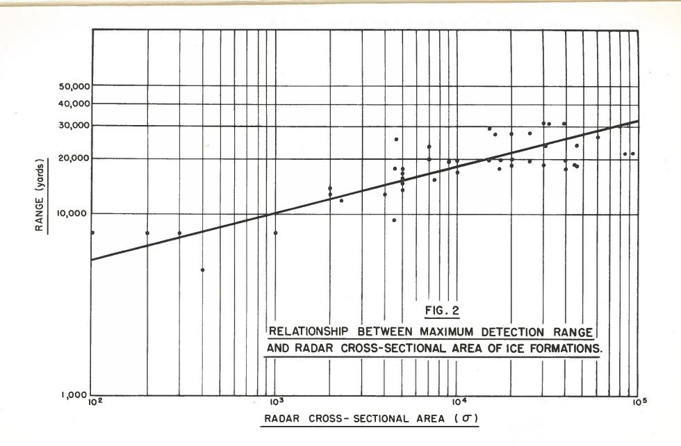
The rated peak power outputs vary from 7 to 26 kilowatts, but this discrepancy does not affect the results seriously, since power output must be increased 16 times in order to double the detection range, R, of a given target.
