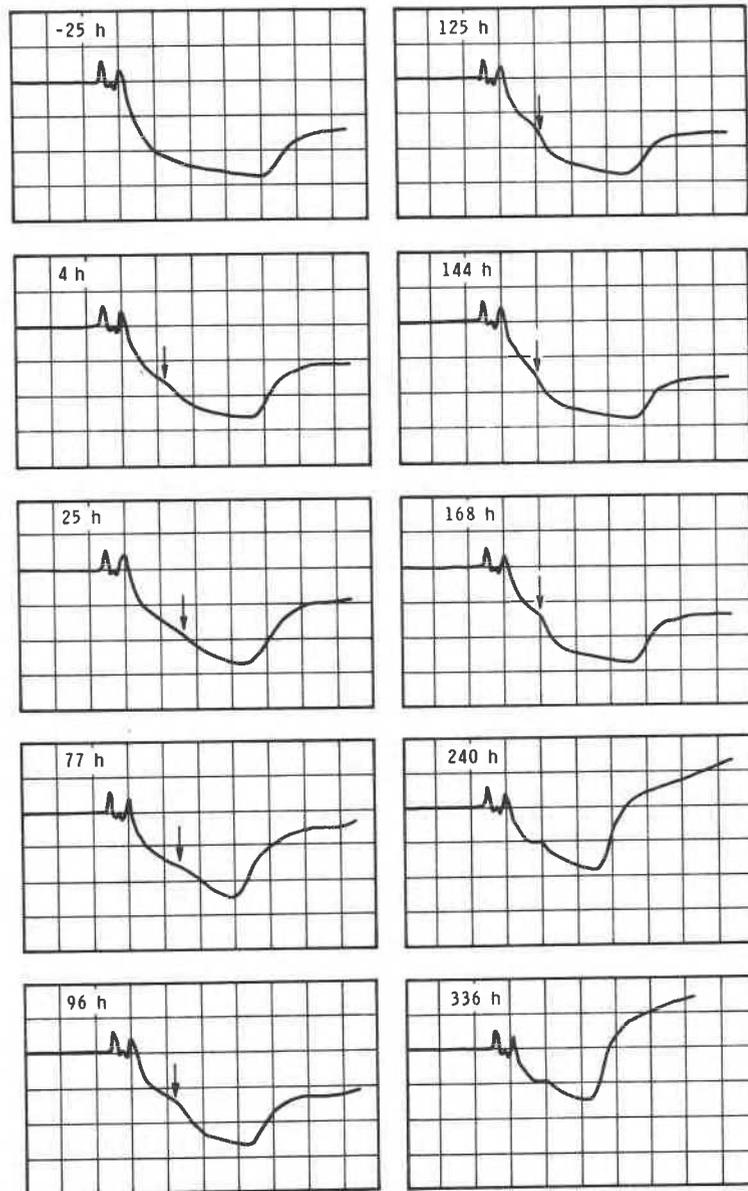
Figure 6. TDR waveforms for the silty clay experiment scale: vertical 200 mp/div; horizontal 2 ns/div
