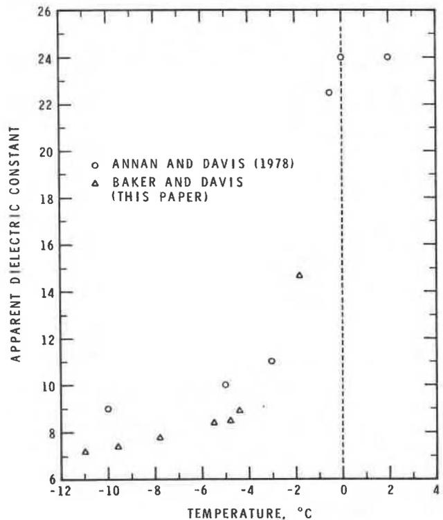
Figure 3. Temperature effect on apparent dielectric constant of silty clay
