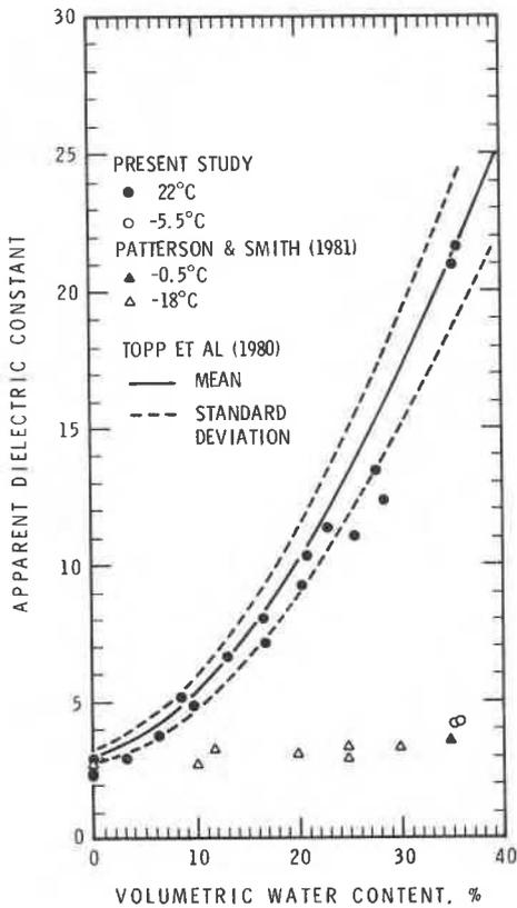
Figure 1. Volumetric water content versus apparent dielectric constant for Ottawa sand at various ambient temperatures
