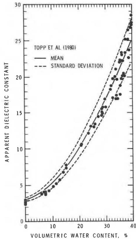
Figure 2. Volumetric water content versus apparent dielectric constant for silty clay at 22°C
