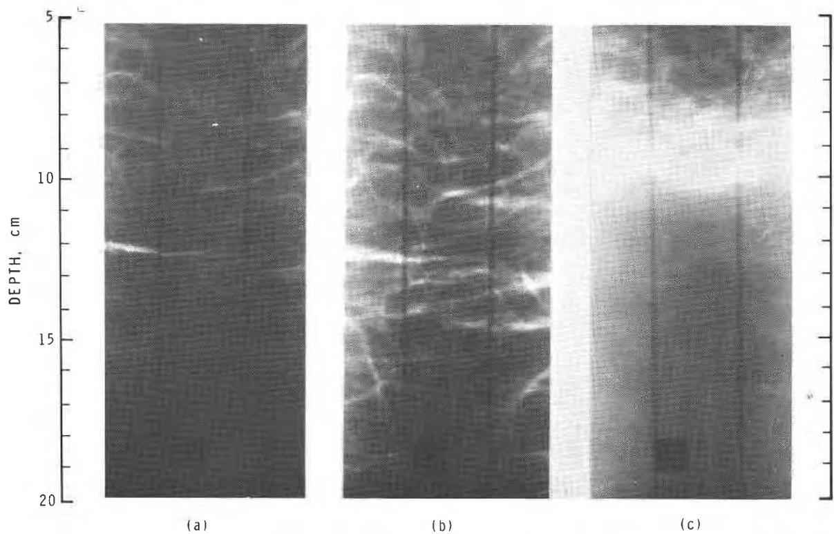
Figure 8. Radiographs from the silty clay experiment, (a) 7.5 hours (b) 79 hours (c) 173 hours
