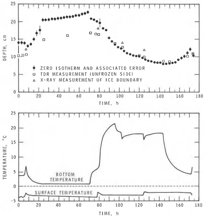
Figure 7. Data from the silty clay experiment
