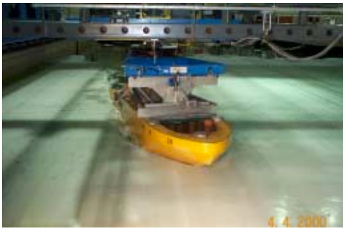
Fig. 7 The PMM Terry Fox Model Test (Lau, 2006)
