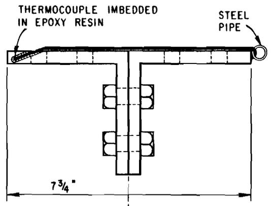
(b) POSITIONING OF THERMOCOUPLES AT 1 FT INTERVALS ON STEEL POSTS IN SECTION
