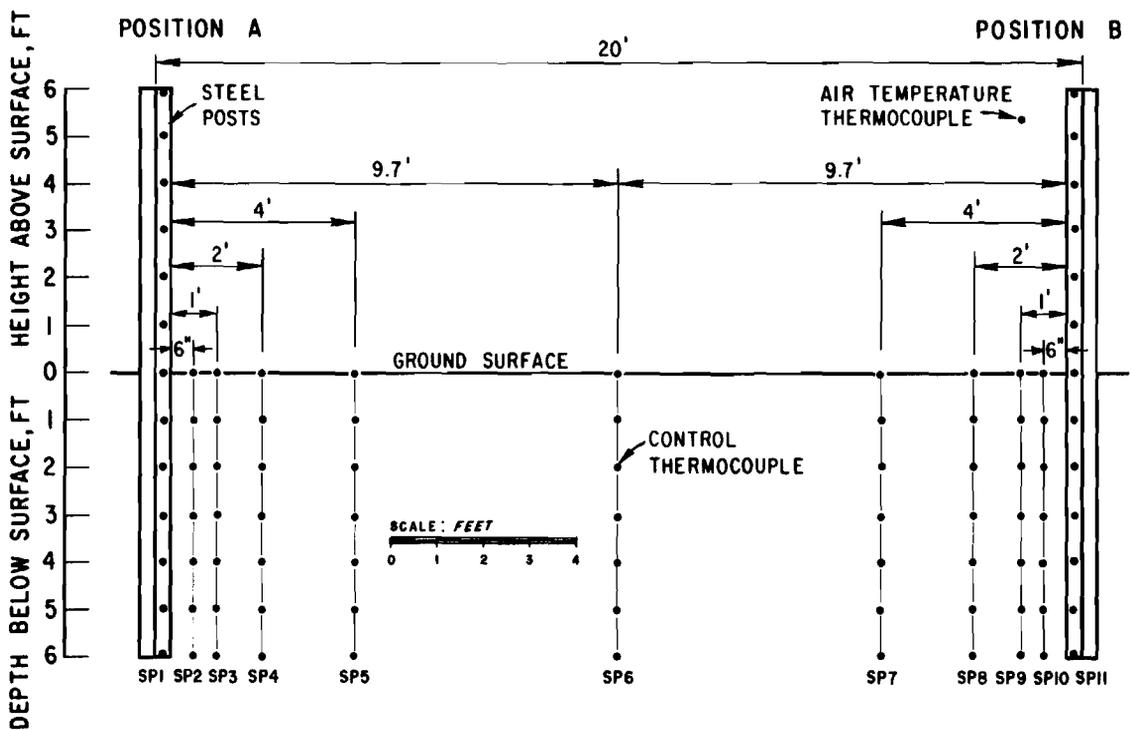
(c) EXPERIMENTAL LAYOUT OF THERMOCOUPLES
