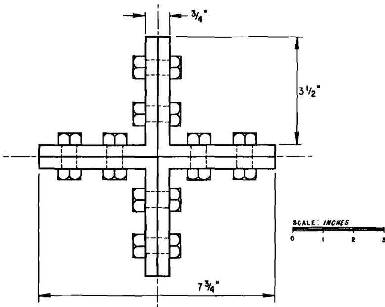
(a) ARRANGEMENT OF STEEL ANGLES IN SECTION
