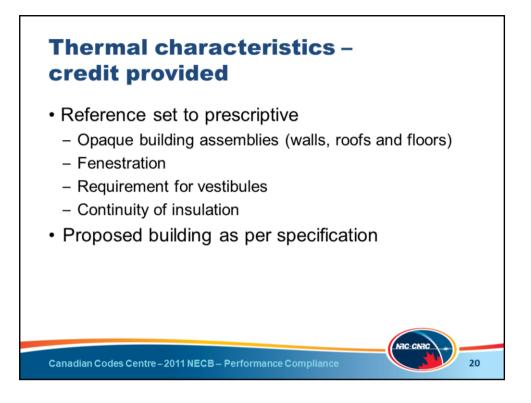
The thermal characteristics of opaque building assemblies (walls, roofs and floors), fenestration, requirements for vestibules and continuity of insulation are modeled as per the prescriptive requirements.
