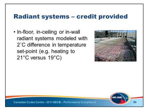
In-floor, in-ceiling or in-wall radiant heating and/or cooling system are modeled with a 2°C difference in temperature setting between proposed and reference buildings, thereby providing a credit in the proposed building. This means the reference building would be modelled at 21°C versus 19°C for the proposed building.
