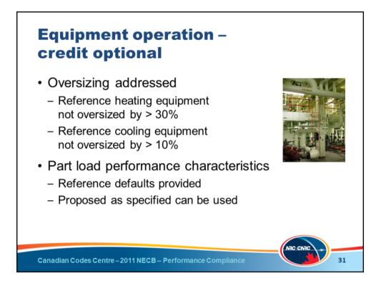
Part 8 addresses equipment oversizing in more detail than the prescriptive requirements. Reference building heating equipment shall not be oversized by more than 30% of the capacity required. Reference building cooling equipment shall not be oversized by more than 10%. The proposed equipment is modeled as specified.
