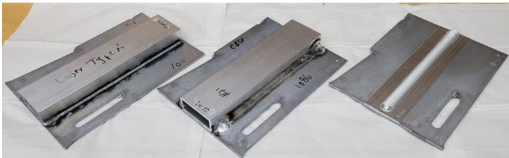
Figure 3: Simple welded assembly specimens from first phase of the project focusing on durability of welded structural castings
