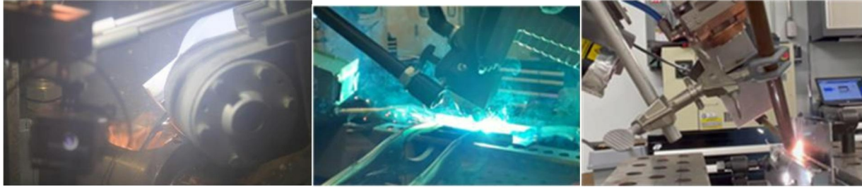
Figure 2: Example of aluminium transformation processes operated at the NRC: high-pressure vacuum die casting (left), gas-metal arc welding (middle) and laser welding (right)
