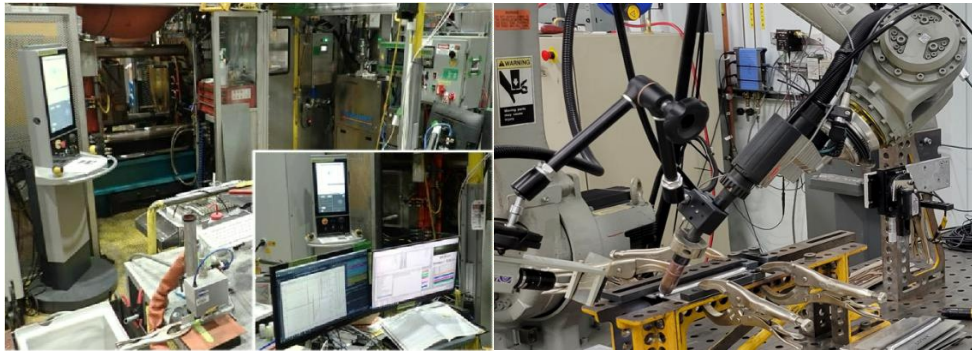
Figure 1: Industrial-grade process cells at the NRC: high-pressure vacuum die casting (left) and robotized gas-metal arc welding (right)
