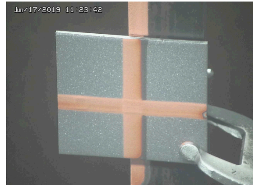
Figure 5. Example of resulting coating corresponding to laser/particle jet positioning (7,-2).
