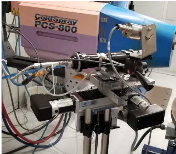
Figure 2. Experimental setup showing the mounted spray gun and laser apparatus on the robot arm.
