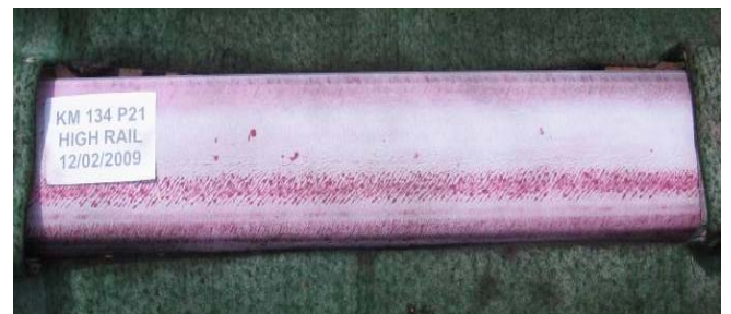
Figure 4 – Dye penetrant for rail surface evaluation
