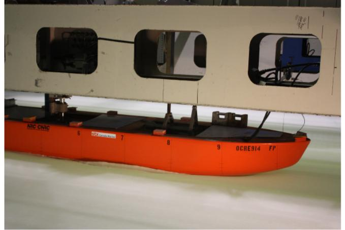
**Figure 3. Towed resistance test in ice**
