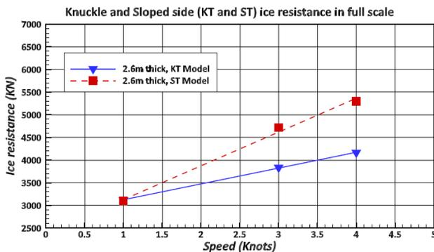
Figure 6. Ice resistance comparison between knuckle and sloped side models
