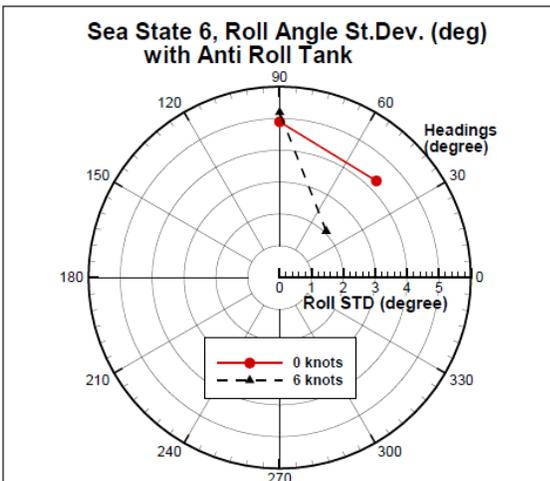
Figure 15. Roll angle standard deviation with anti-roll system
