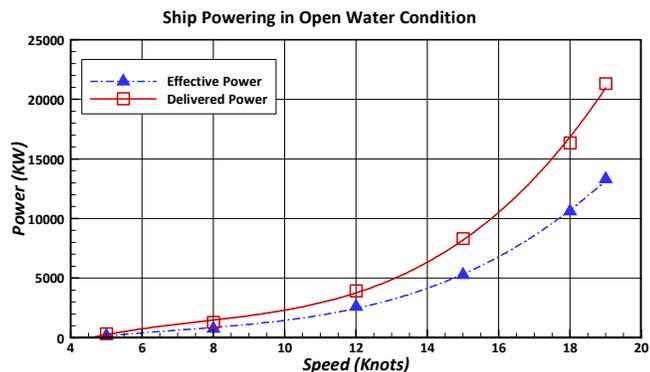
Figure 18 Ship powering in open water condition
