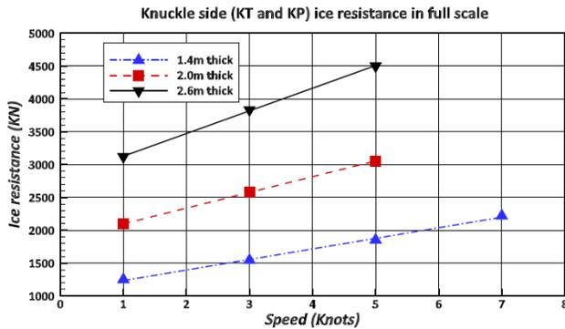
Figure 5. Ice resistance for the knuckle side mode
