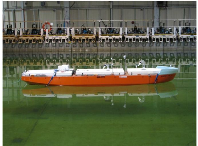
Figure 17. Stationkeeping test
