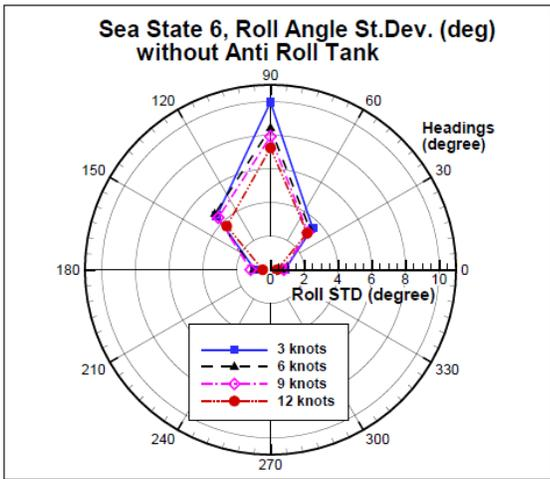
Figure 14. Roll angle standard deviation without anti-roll system
