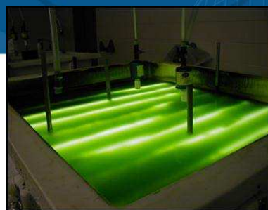
1000 L Brite Box, lid removed showing microalgae culture
