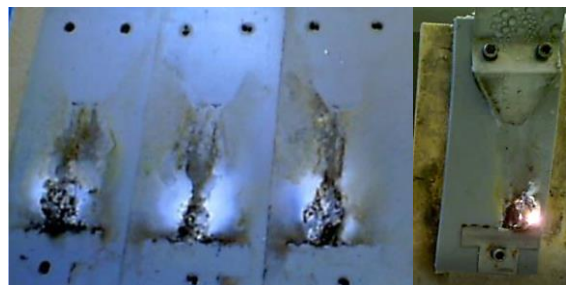
Figure 2. Failed silicone rubber composites containing 25 wt% ATH under DC voltages due to combustion/erosion paths.
