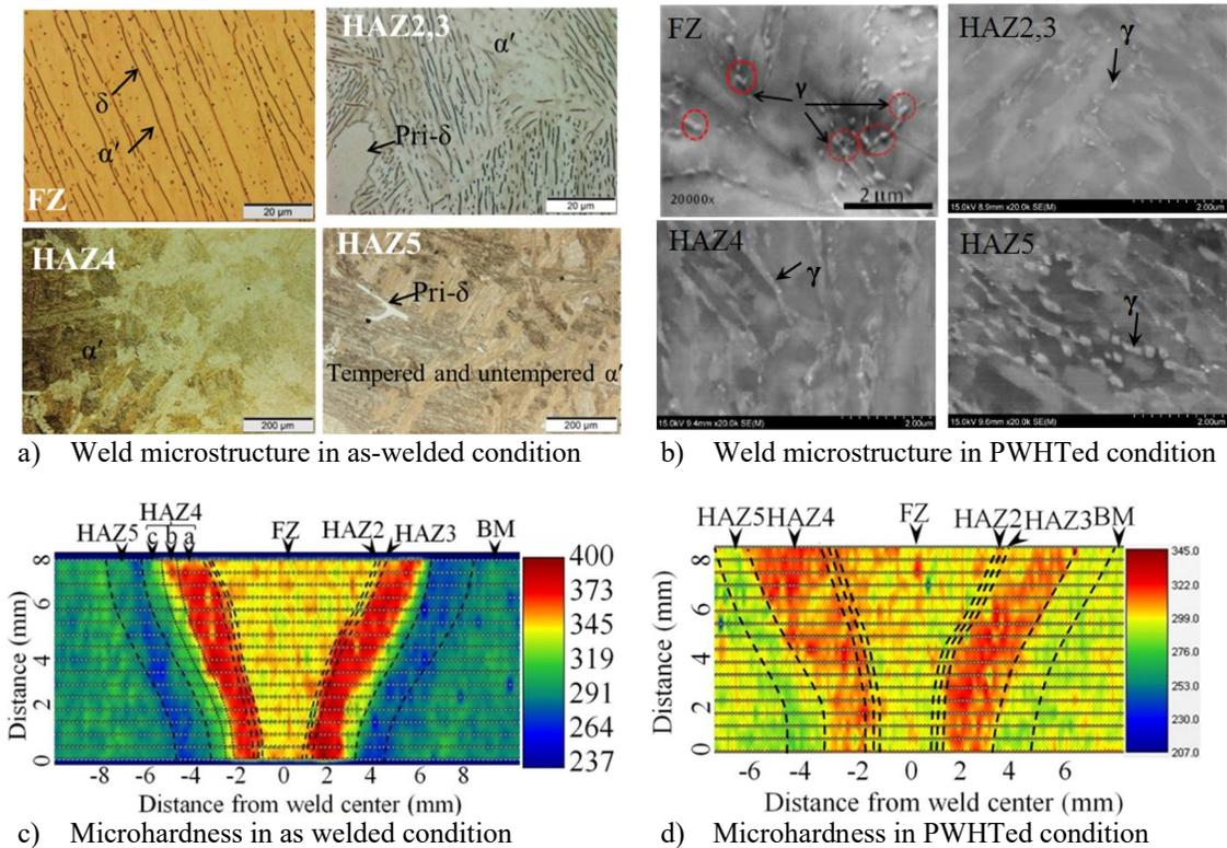
Figure 2. Microstructure and microhardness in as-welded and post-weld tempered conditions
