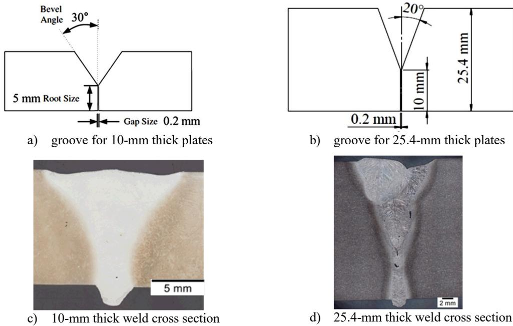
Figure 1. Groove design and weld cross sections for the two plate thicknesses
