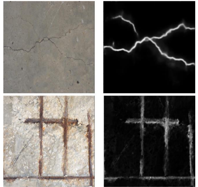
Figure 4. Early images of defect segmentation using U-Net.
