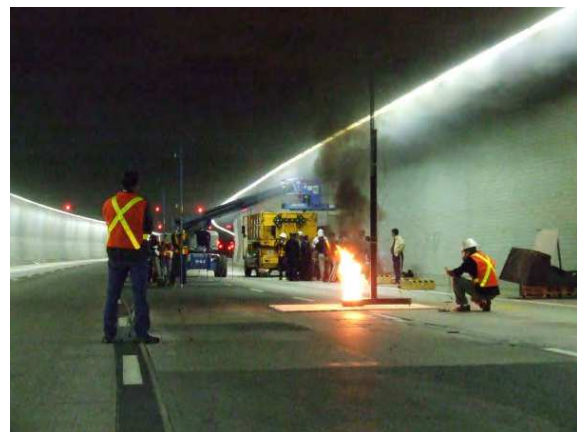
Figure 3. Fire tests in a Montreal operating tunnel
