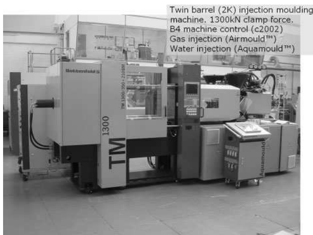
5 Battenfeld injection moulding machine with separate gas/water injection controller shown in foreground; water injection reservoir is shown behind machine
