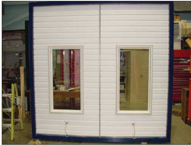
Figure 2. (a) Sample wall-window test assembly; (b) Diagram of wall-window assembly showing locations of wall-window interface details
