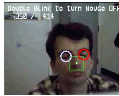
Fig. 6. Using double-blink to switch Nouse on/off.
