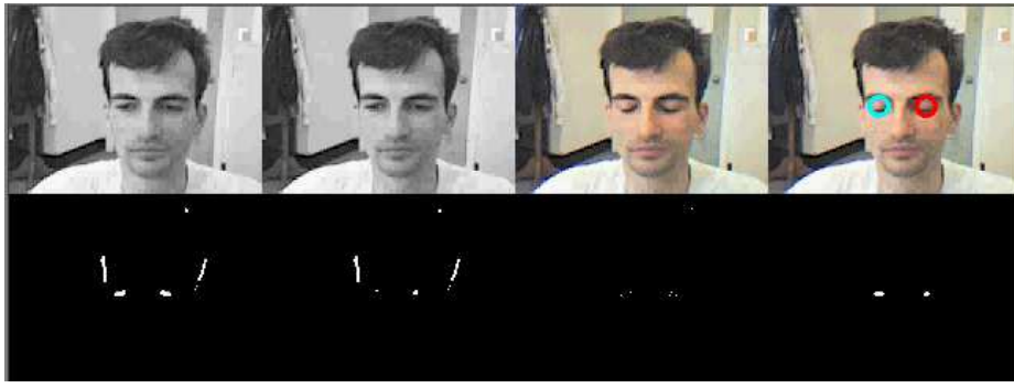
Fig. 4. Detecting eye blinks using the second order change detection. The pixels changed because of head motion removed by the second order change detection procedure are shown at the bottom center images. See also Figure 2.
