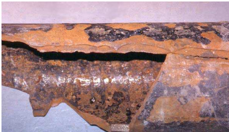
Figure 3. Longitudinal split following corrosion initiated by scratch in coating (Ottawa, 1998).
