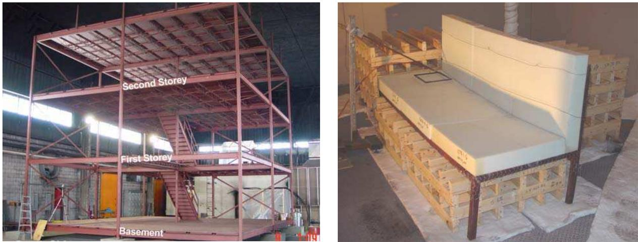
A fuel package representing a sofa fire was developed to create a repeatable fire in the basement. The first item ignited was polyurethane foam which ignited a wood crib, see Figure 3. This produced a relatively severe, fast-growing fire generating CO and CO<sub>2</sub> in a vitiated oxygen environment. The floor assemblies were tested under two conditions: with the basement door open or closed.
