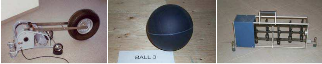
Figure 1 – Standard impact sources. From left to right: Bang Machine (Tire), Ball, ISO Tapping Machine (Hammer). Detailed descriptions of sources can be found in the following standards: Tapping Machine: ISO 10140-3, JIS A 1418-1, KS F 2810-1; heavy impactors: ISO 10140-3 (Ball), JIS A 1418-2, KS F 2810-2.
