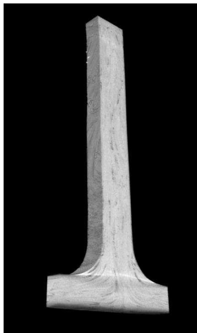
Figure 8. Micro-CT rib three-dimensional rendering.
