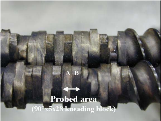
Fig. 18. The probed screw type and area under the monitoring of the clad buffer rod probe shown in Fig.17.
