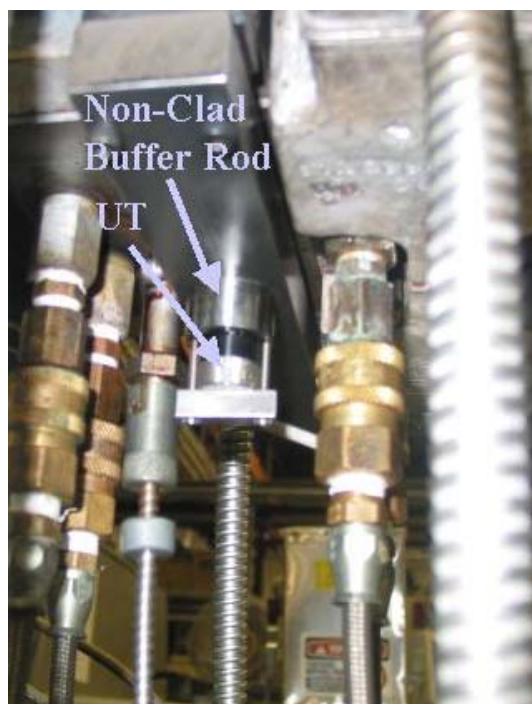
Fig. 11. A non-clad buffer rod probe mounted at the bottom of a barrel at the mixing zone with the help of a holder. The heating band did not cover the bottom surface of the barrel.
