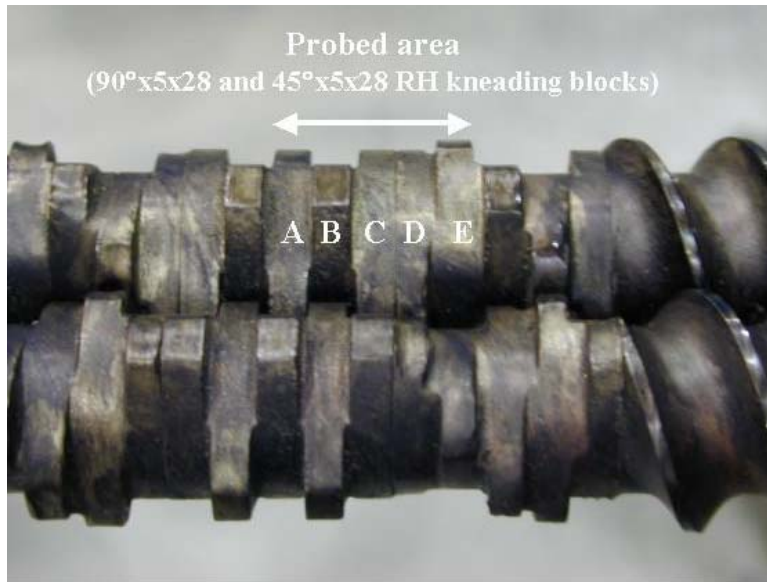
Fig. 12. The probed screw type and area under the monitoring of the probe shown in Fig. 11 at the mixing zone.
