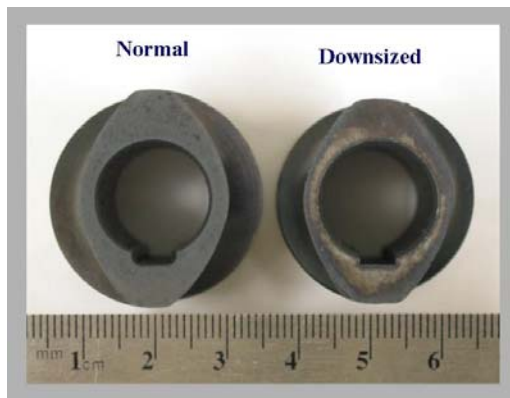
Fig. 8. The screw bushings (28/28 RH) probed in setup of Figure 7.
