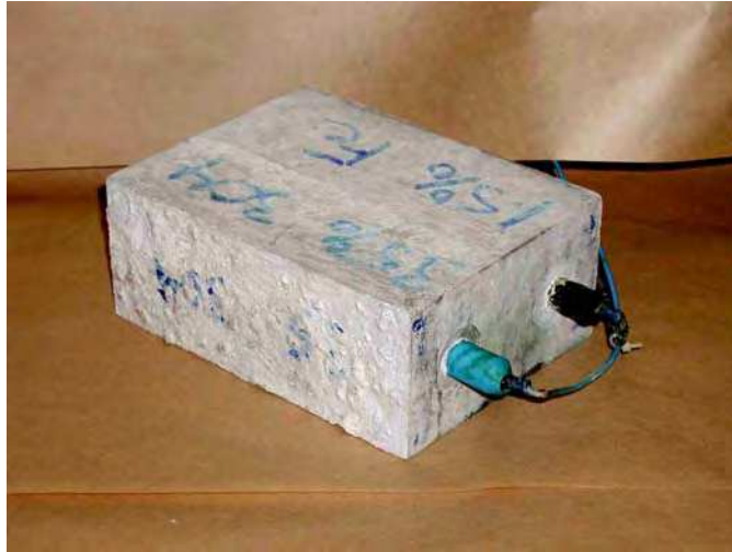
Figure 2. - Photo of a concrete specimen used in galvanic coupling tests
