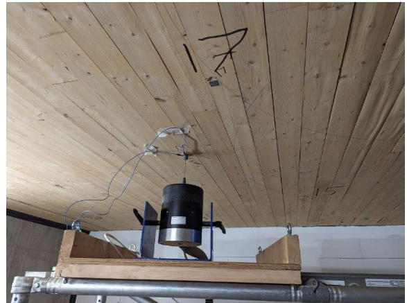
Figure 4: A 100 N shaker attached to the CLT ceiling. An impedance head attached to the stinger allows for the measurement of the mobility.
