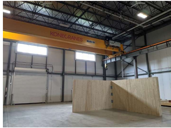
Figure 5: A mock cross-junction between two CLT walls connected with brackets spaced 400 mm on center. The mock-junction is located in a new K_{ij} measurement area with an isolated floor. A layer of resilient material is located between the elements and the floor.
