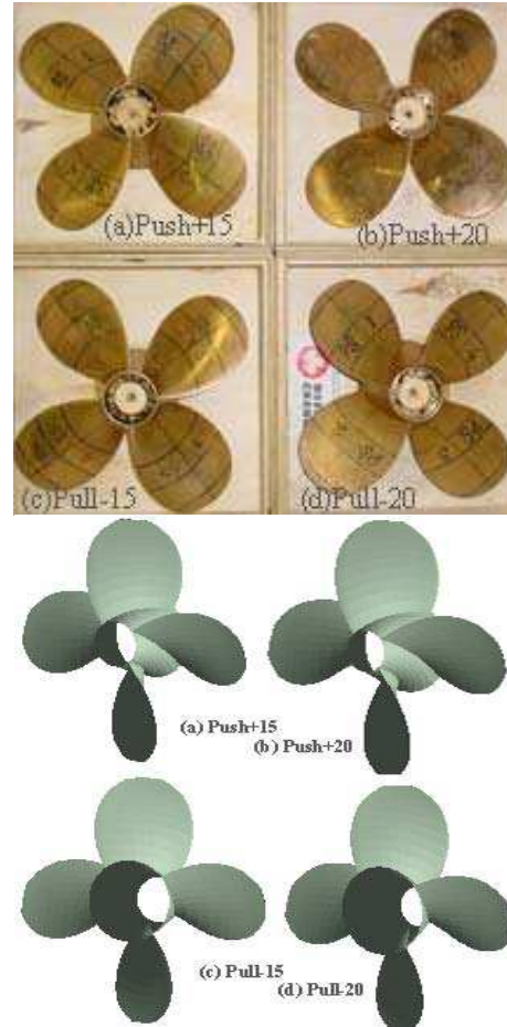
Fig. 5 Four model propellers (Top- actual physical model; Bottom- rendered model). Figure (a), (b), (c), (d) are the propellers with hub taper angles of +15^\circ (push), +20^\circ (push), -15^\circ (pull), -20^\circ (pull), respectively.
