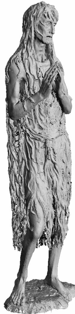
**Figure 3. Complete model of the sculpture. lateral resolution: 0.25 mm and depth uncertainty:  $\sigma_z=70$   $\mu$ m**
