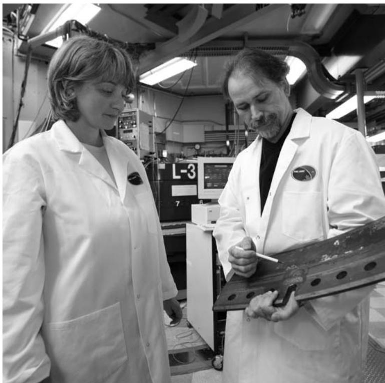
NRC scientist Dr. Ron Rogge explains to post-doctoral researcher Roxana Hutanu how, as part of the Challenger accident investigation, neutrons were used to measure the stress inside this component from NASA's space shuttle.
