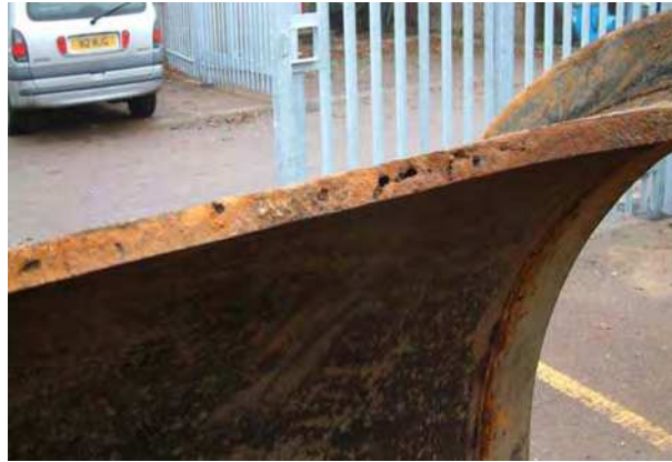
Figure 3. Typical casting voids and defects in small and large diameter grey cast iron pipes.
