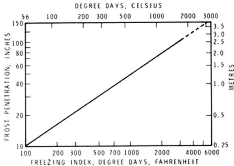
Figure 2. Relation between Freezing Index and depth of frost penetration (Brown, 1946).
